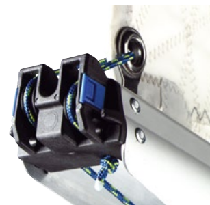
Outboard end Lines can be locked via two pegs on the side of the fitting or via a V-groove underneath the starboard sheave.
