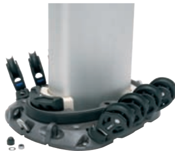
Step the mast and replace the wedge.
