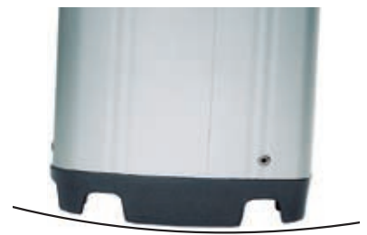
Convex underside of heel plug – distributes compression load evenly on the mast section.
