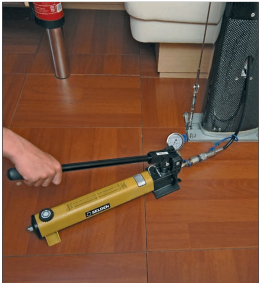
...and can easily be fitted to the pump to adjust the rig tension.
