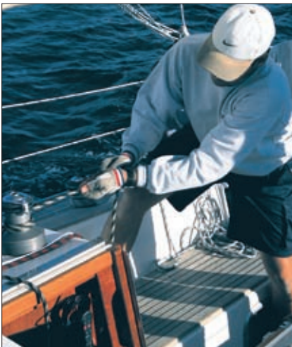
Tension the reef line up to the marked position on the line.
