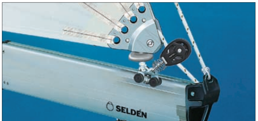
Boom fitted with outhaul car for Seldén furling mast. For hydraulic outhauls, see page 103.
