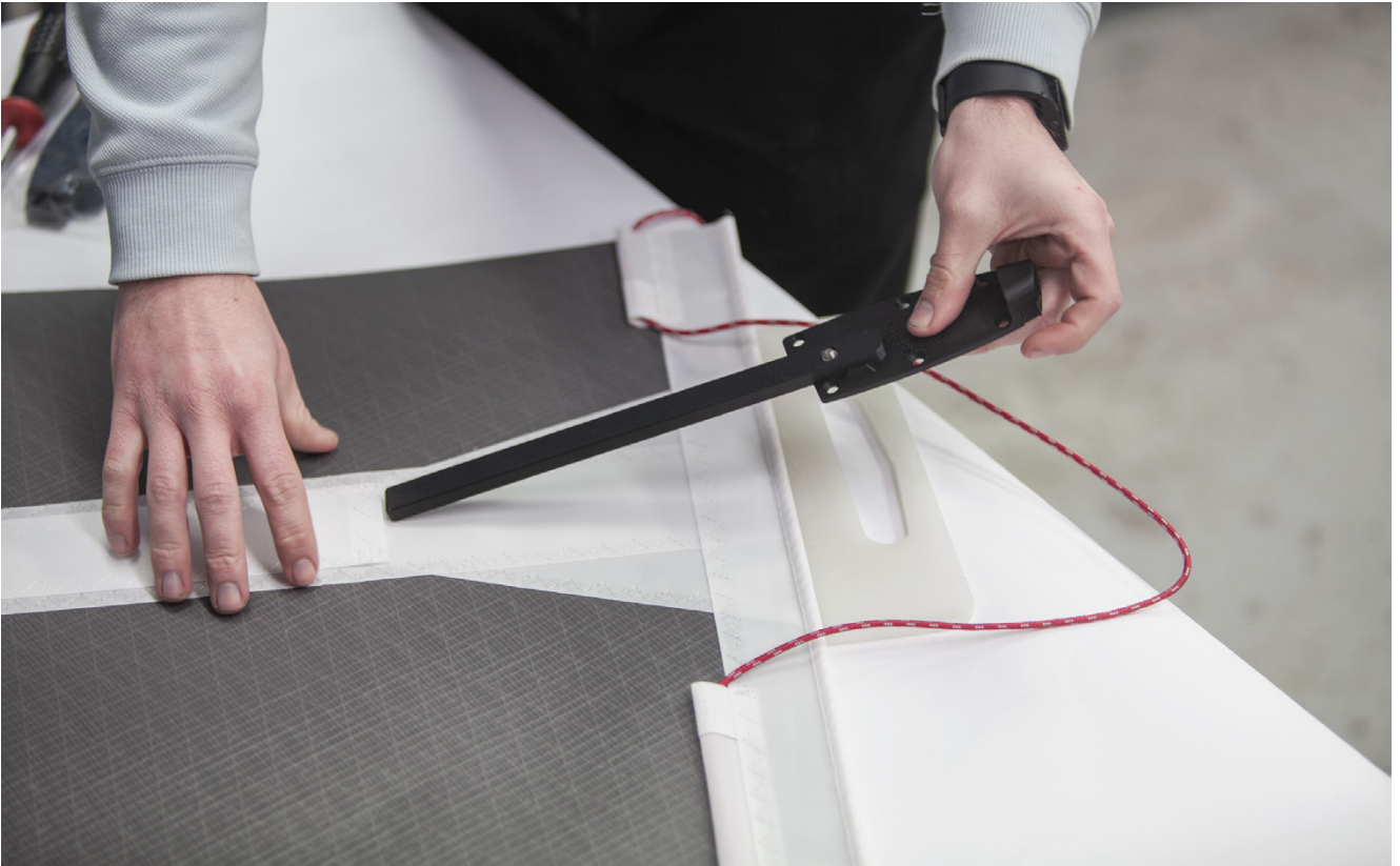
3D template for attaching batten receptacles
