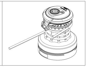
Gently ease the tension in the pulling end to induce slipping over the winch drum, releasing the tension in the sheet.
