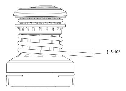
To achieve the correct angle, installing a block or sheet lead to divert the sheet or halyard to the winch may be necessary. Please visit www.seldenmast.com to browse our selection of suitable deck hardware.
