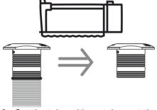
8. Cut the tube with metalsaw at the mark
