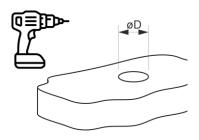
4. Drill a hole in the deck according table 2
