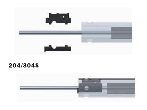
Fit the bearing halves in the lower extrusion as shown. Secure halves with the spring pin (A).
