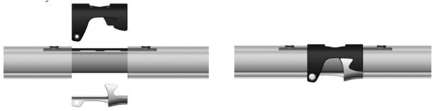
10. Fit the halyard swivel from the top and slide it down until it stops on top of the sail feeder. Then fit the top guard and push it into the top luff extrusion until it stops. Secure it with the two pre-fitted screws. Tighten the screws until they bottom, but do not over-tighten.
