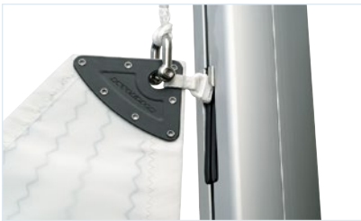
1) Feed all sliders into the sail entry.
