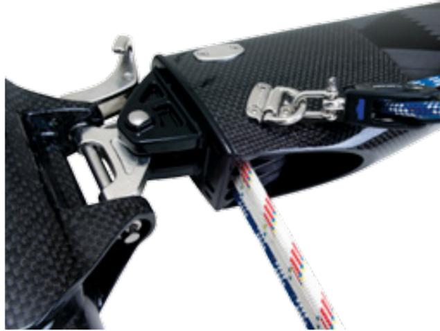
The outboard end features an alloy sheave housing which is again integrated in the main tube and is concealed from view by a carbon coverplate across the boom end.
