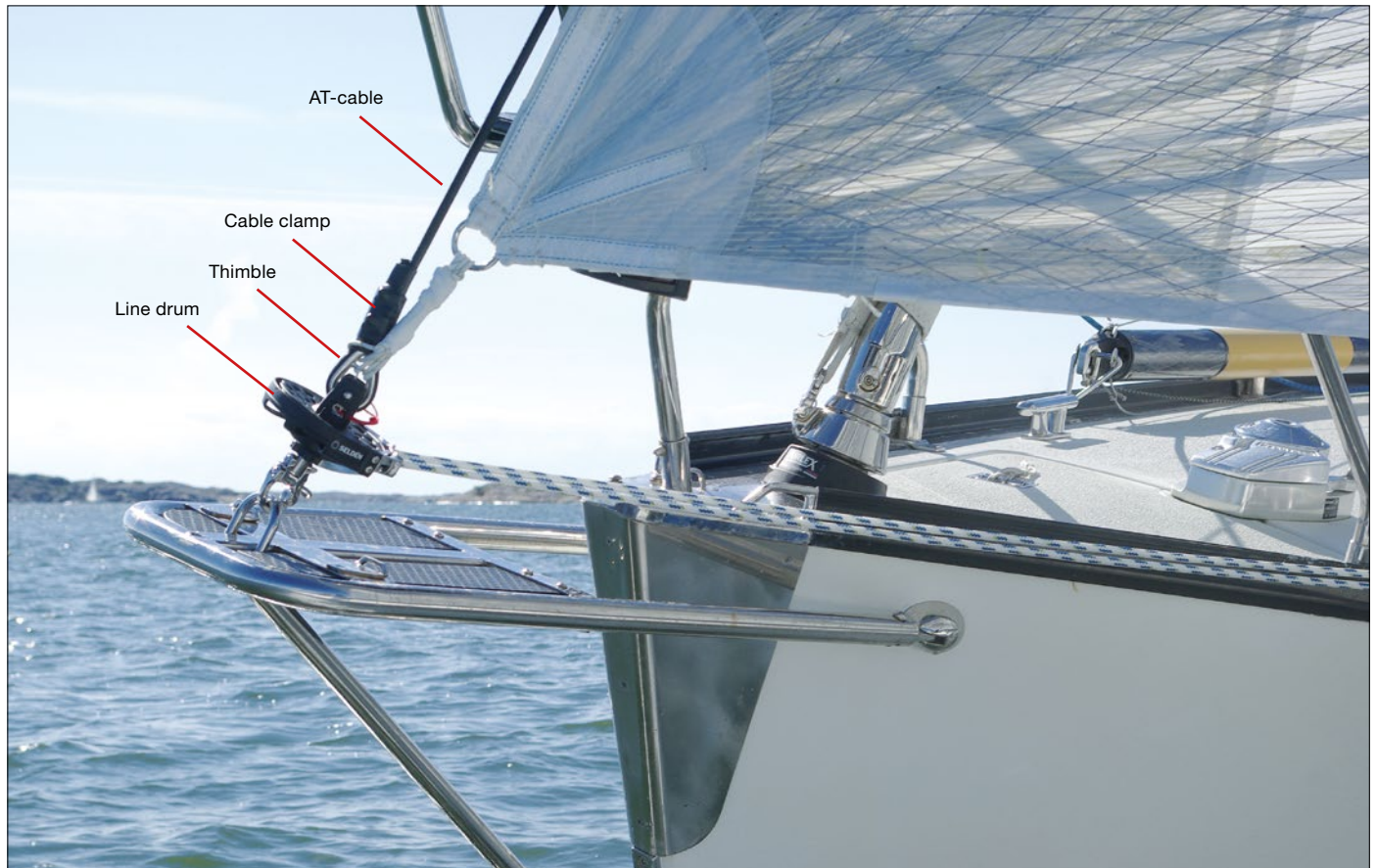
A Seldén CX15 Code 0 furler and a Race80 Bowsprit from Båtsystem, Sweden. www.batsystem.se . The luff load on a Code 0 is more than the double compared to an asymmetric spinnaker. Therefore, a sturdy bowsprit is required.
