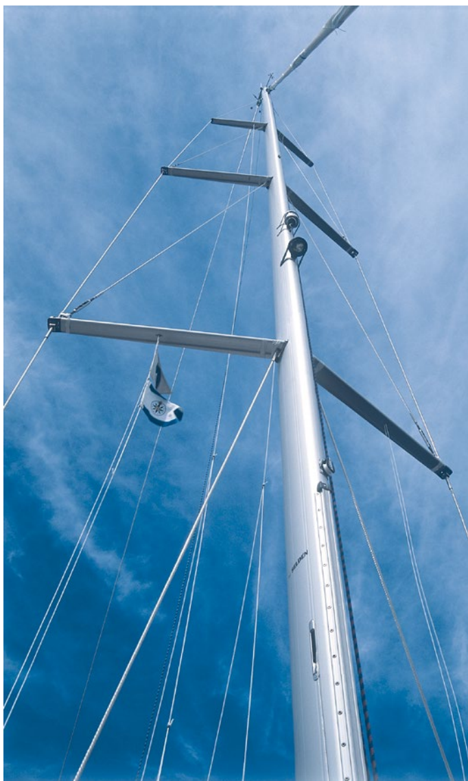
Seldén T-spreaders for C-sections and F-sections.
