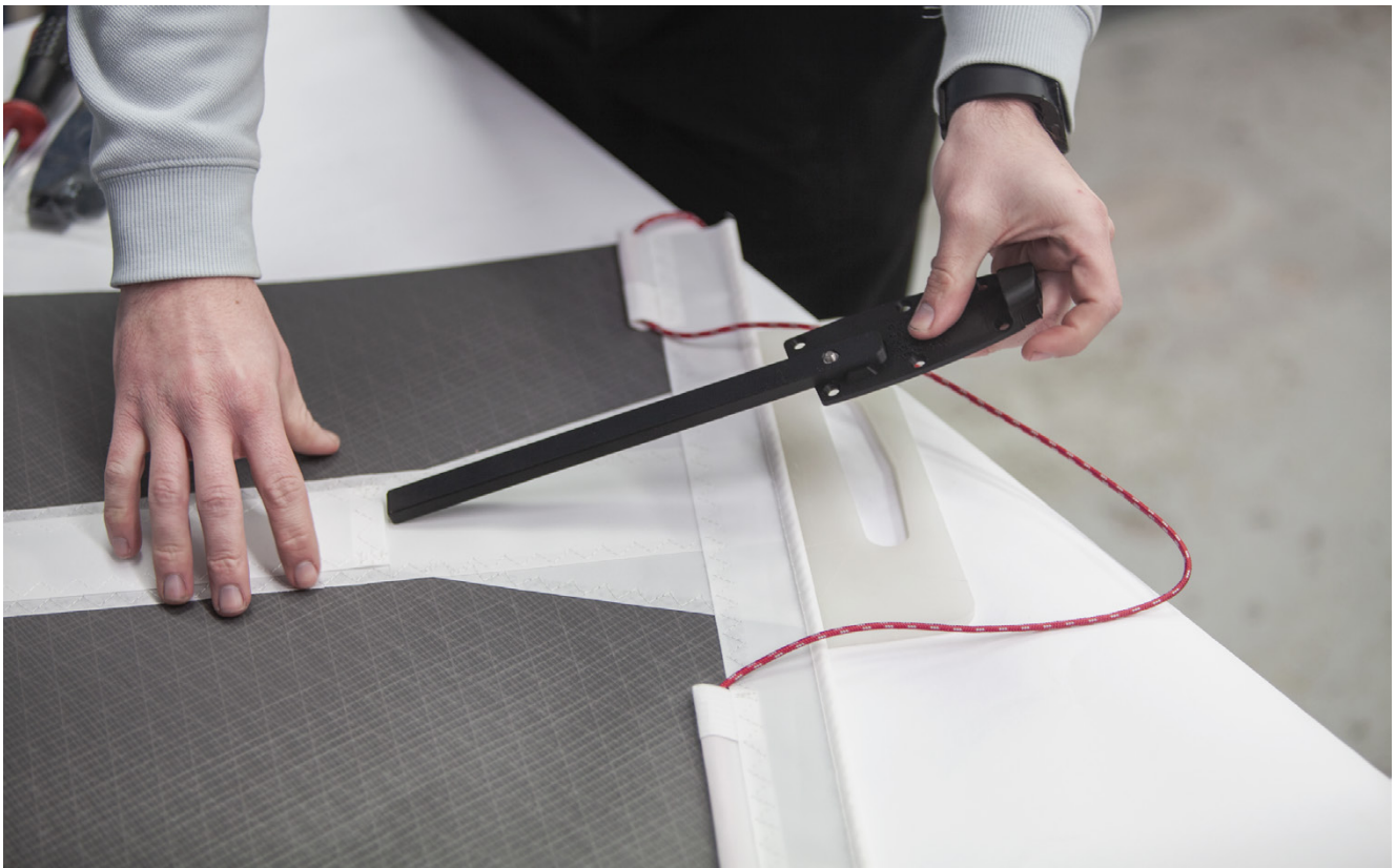
3D template for attaching batten receptacles
