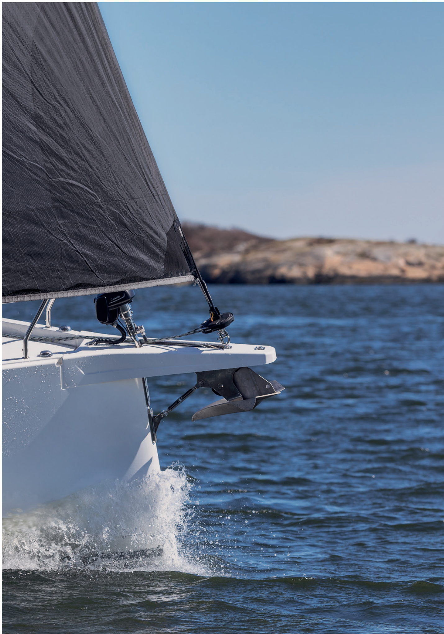
CXr furler on a bowsprit. Connected to a fixed folding pad-eye.
