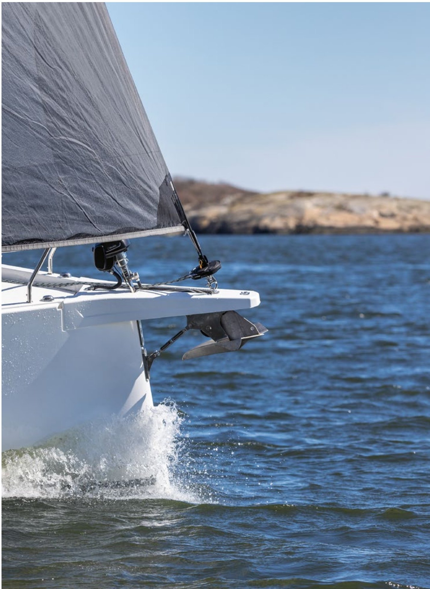
CXr furler on a bowsprit. Connected to a fixed folding pad-eye.
