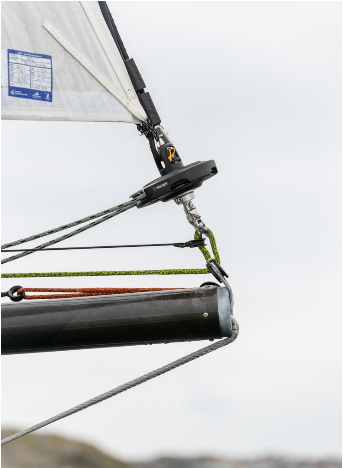
CXr furler on a retractable carbon bowsprit. The low friction shackle (optional) underneath the drum is connected to the tack-line. 2:1 purchase enables the bowman to pull the drum out on the bowsprit while remaining on the foredeck. It also makes for a high luff load.
