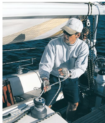
If necessary, apply more main halyard tension.
