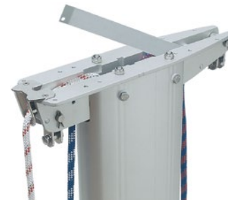
Separator locks sheaves and also controls spinnaker halyard.
