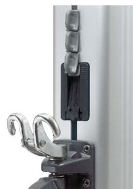
Sail entry gate designed for use with Seldén MDS cars or conventional sail slides. For detailed information about our conventional sail slides, please see Sailmakers Guide, www.seldenmast.com .
