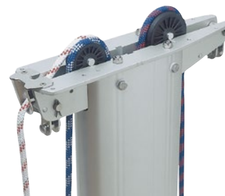
Top access, without unstepping the mast and removing the headbox.
