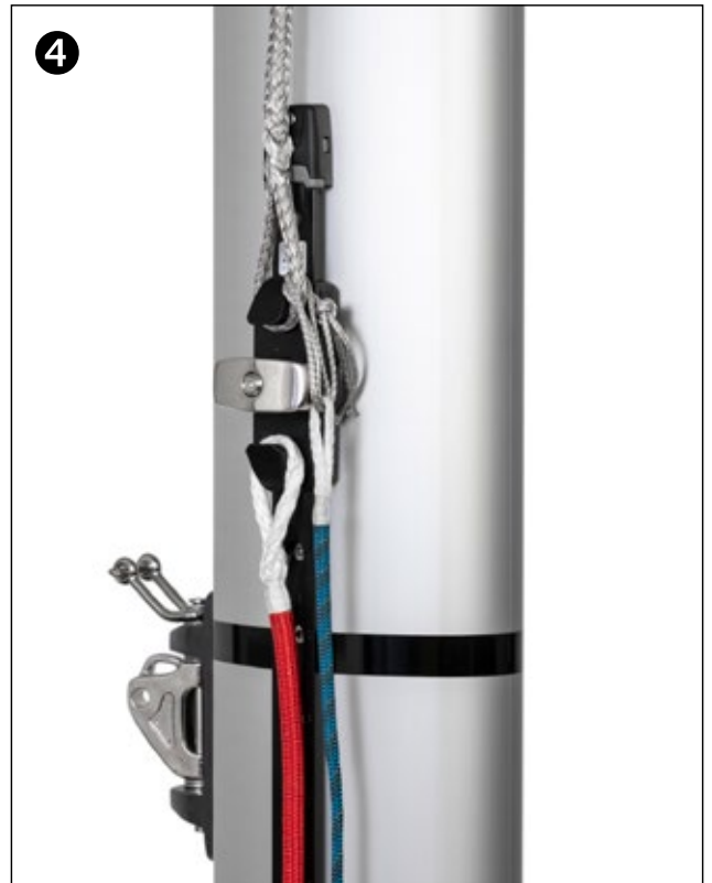
4. Attach a tail-line to the lower bucket and lead it to a winch. Twist the handle to the closed position.
