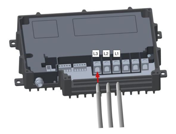
CXe comes with three black cables to be positioned in connectors L3, L2 and L1 in no particular order.
