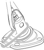
**CXeTD**: Connect a suitable strap between the loop in the deck collar and the thimble or fork.
