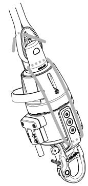
**CXeOD**: Connect a suitable strap through the bracket and the thimble or fork.
