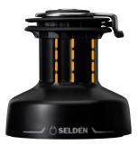
The drums we are using for our new manual and electric winches are forged and machined hard anodised aluminium with vertical ribs located in an asymmetric pattern. Any line under load will become slightly dented where it rests over a rib and if all ribs were located symmetrically, all dents would simultaneously jump to the next rib when releasing the line. And the next one, and the next one...
