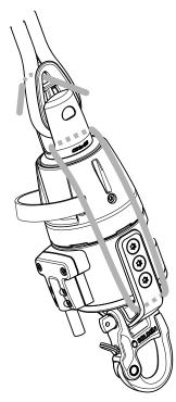
**CXeOD**: Connect a suitable strap through the bracket and the thimble or fork.
