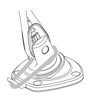
**CXeTD**: Connect a suitable strap between the loop in the deck collar and the thimble or fork.
