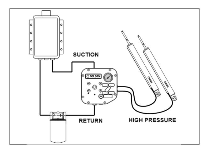
Hose layout example with four function pump station, two functions used
