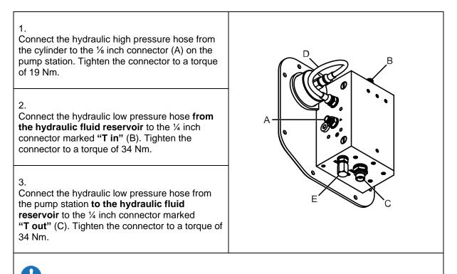
**ATTENTION!** Perform the connections cautiously so that the hose (D) to the pressure gauge is not squeezed!
