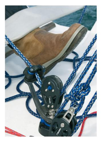
**Horizontal articulation.** The angle of horizontal movement is easily adjusted without taking the swivel apart. Two stops can be fixed in 5 different positions, from a fixed arm to 300° angle of movement.
