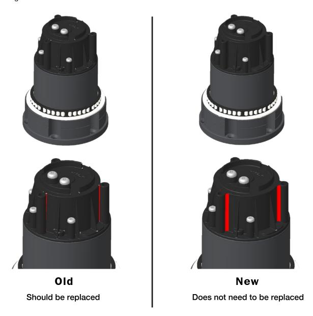
If the radii marked in red are small as in the pictures to the left the cover should be replaced, according to this manual. If radii marked in red are large as in the pictures to the right the cover is already the latest version and does not need to be replaced.d
