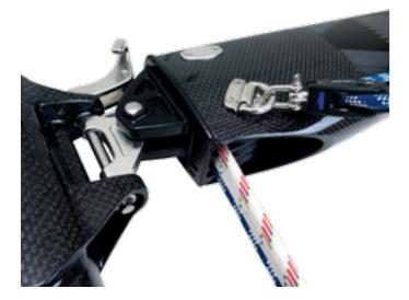
The outboard end features an alloy sheave housing which is again integrated in the main tube and in concealed from view by a carbon coverplate across the boom end.
