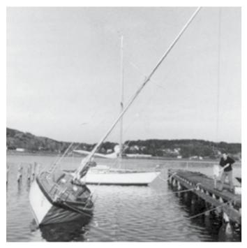
Heeling test in 1965. The righting moment of the boat is measured ay 30° heel.
