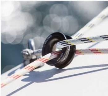
One ring used for gennaker sheet and Code 0 sheet.
