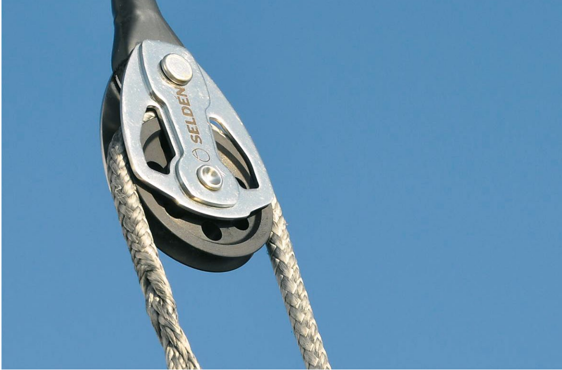
Dyneema core in the bridle is an alternative to 7x19 strand wire.
