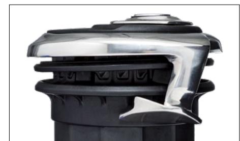
*The groove of the self-tailer does not have the traditional wedge shape but is a round cavity encircling the line. A spring loaded disc provides just enough pressure to keep the line in place. The feeder arm is highly polished stainless steel.*
