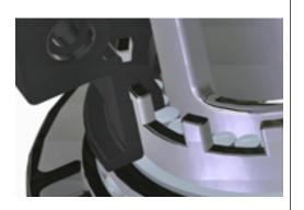
6. Fit the four self-tapping screws-ensuring not to over tighten. Do not lift assembly during this operation. Re-assemble bearing ring, balls, washer (+any shim) and the new retaining ring. Make sure retaining ring engages groove properly. Grease balls before fitting washer.
