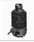
3. Find the end of the 2-turn retaining ring, lift out of the groove using a small screwdriver or knife. Work around the shaft until the ring disengages from the groove completely. The ring can now be pulled off the shaft by hand. Use a screwdriver if the ends catch the holes in the shaft. Remove shim (if any), washer, balls and bearing ring.
