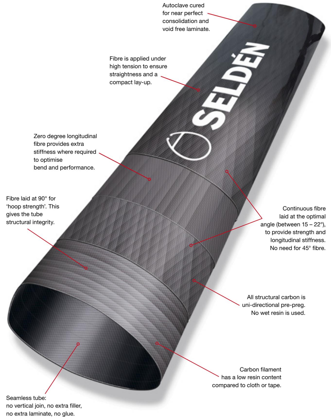
Autoclave cured for near perfect consolidation and void free laminate.
