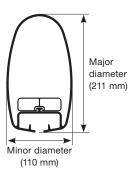
Mast section measurements are given as follows: Major diameter/Minor diameter (i.e. 211/110). This will help identification and the use of correct measurements. The major diameter of the mast can usually be found in the number engraved at the mast heel. For example K23-C211-4475.
