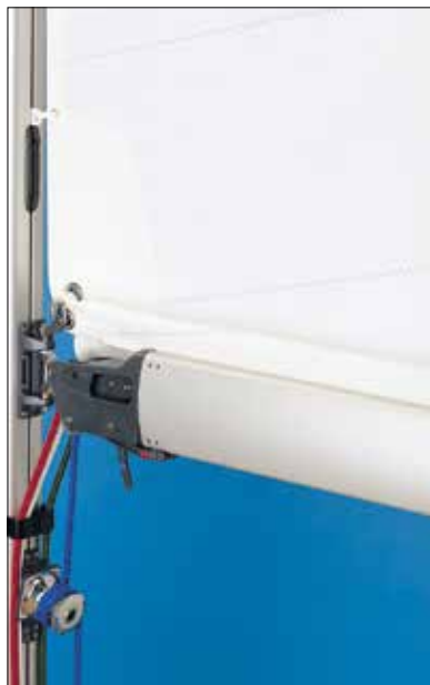
Slab reefing with fixed hooks.
