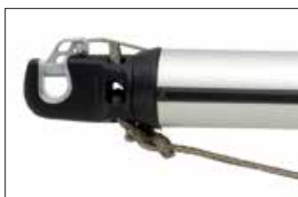
Composite spinnaker pole fitting, Art. No. 534-865.
