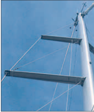
Seldén T-spreaders for C-sections and F-sections.
