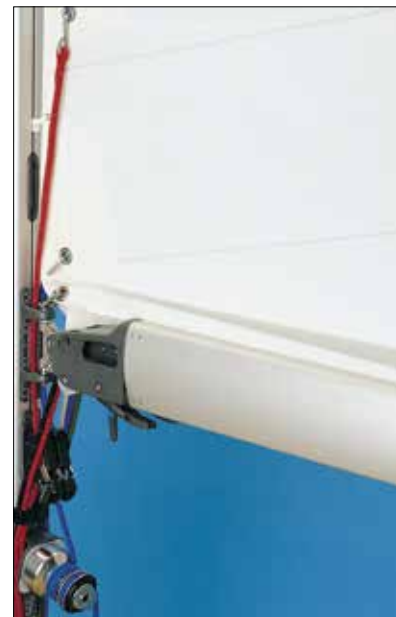
Slab reefing with running S-hooks.
