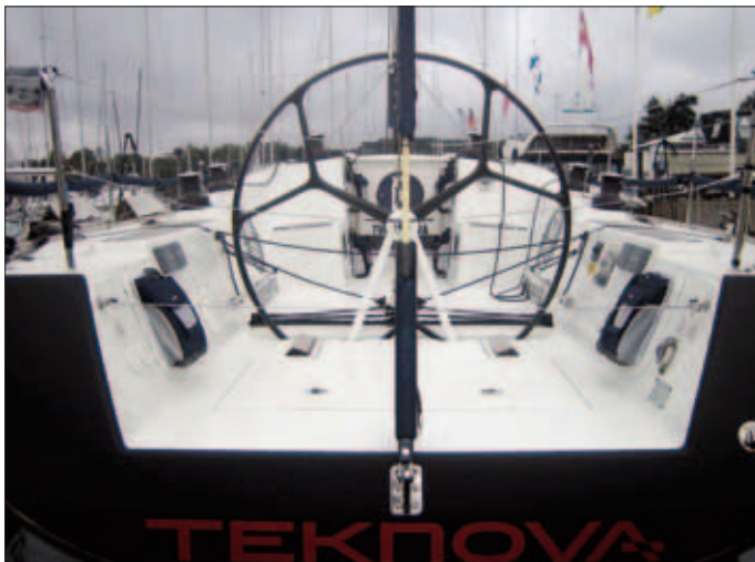
First 40 featuring a HT-W8/10 tensioner and control panels both sides in the cockpit.
