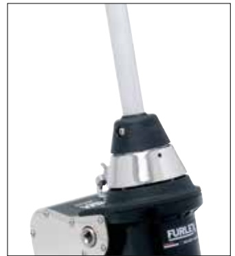
Slide on Furlex 200E from below and install the cables. Done!
