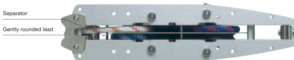
Masthead headbox for C211-C301 and F212-F406. The headbox fitting has a gently rounded lead for a masthead spinnaker and gennaker. The separator is slightly angled at its front end to lead the halyard on to the sheave.
