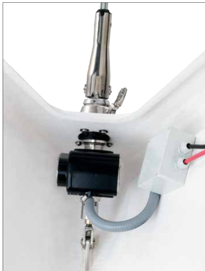
Installation of a Furlex 200TDE. The connection box is water-tight.
