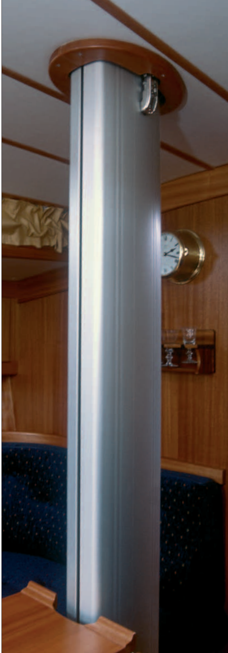
Deck ring with moulded mast coat.
