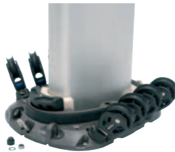
Step the mast and replace the wedge.
