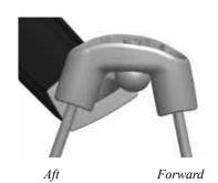
Put the threaded M10 bars into the bracket 443-200. Use the bars to find a good location for the deck fittings.
