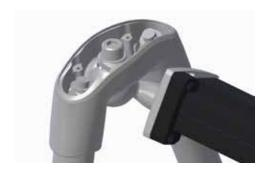
Fit the two lids with M4 screws.
