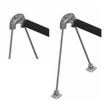
Fit the center consoles in the track, drill holes Ø8.5 in the track, insert washers and nuts in the groove of the track
