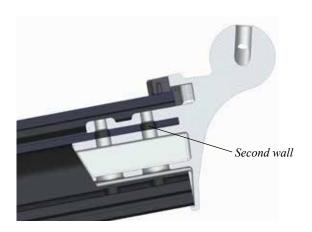
Put the car onto the track and fit the 443-201 on the track. Use Locking adhesive on the screws.
