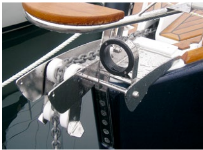
Bow bracket integrated with bow anchor fitting.
