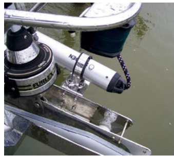
Side mounted installation on stem head anchor fitting.
