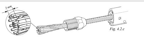
Slide the wedge over the core (7 strands) of the wire . The core of the wire should protrude approx. 3 mm (1/8") from the wedge.
