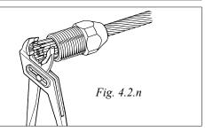
12. Insert the former into the threaded hole of the terminal part (or rigging screw). Lubricate the socket's thread with a long bead of locking adhesive. Screw the terminal part onto the socket and tighten carefully, forcing the wire further into the terminal.
