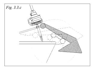
If a custom made extension link is used it must always have a toggle between it and the boat's forestay attachment.
