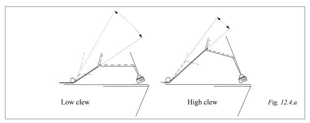
The angular variation of the sheet relative to the deck is less for a high-clewed sail. The comparison is based on the same number of furling revolutions.
