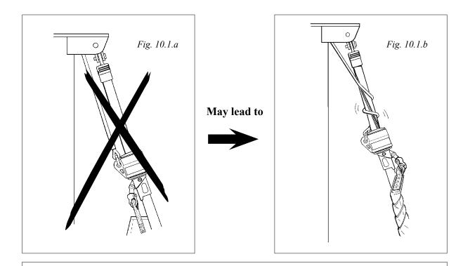
When sailing, movement occurs between the wire halyard and the halyard lead. To prevent halyard wear, the halyard lead is made of bronze. This is a softer material than a wire halyard, so the halyard lead will wear before the wire. Halyard leads should be inspected once a year and any sharp edges smoothed with a file. The halyard lead should be replaced when wear reaches 50%. The halyard leads are not covered by the 2 year Furlex warranty.
