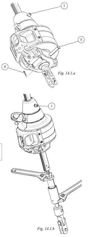
The rigging screw has a stop at the maximum position to which it can be unscrewed. Do not overload this stop by trying to unscrew the rigging screw further with the tool. The values given in the table below for adjustment must not be exceeded!
