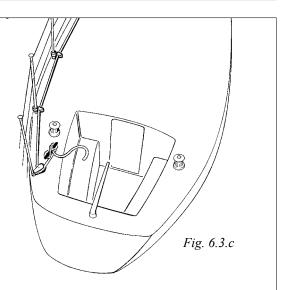
The furling line is best belayed on a cleat. If a stopper is used, its maximum working load must not be less than 50% of the block load.
