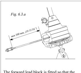
The forward lead block is fitted so that the furling line is straight when it exits the line guide fitting.
