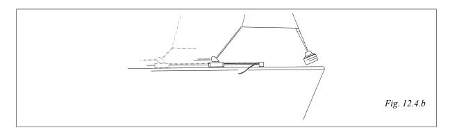
Many furling foresails have markings in the foot for different reefing positions. After you have tested combinations of sail area and sheeting position to see which function satisfactorily, you can use these markings as a reference and mark suitable sheet points on the track.
