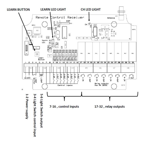
1-2 Power supply: to be connected to 12 - 24V
