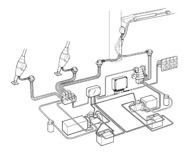
The picture above shows an installation example where the four function receiver box is used together with pushbuttons.
