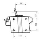
Cross beam be supported by compression beam:
