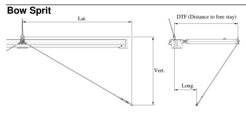
Geometry for bow sprit: All measures are in reference to the fore stay chain plate
