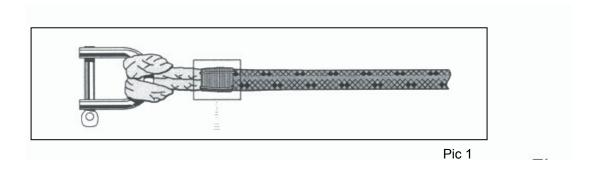
**Design:** Determine how large the eye should be. As little as possible of the core should be visible when the splice is looped around a shackle, see pic 2. After a few trial splices, the size of the eye can be determine easily.
