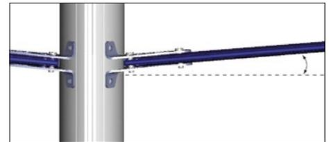
*The new system has the dihedral angle locked into the bracket to give the optimum rig support.*
