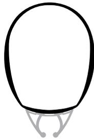
The aerofoil shape of the profiled section also gives improved air adhesion compared to round tubes. So the spar directly increases lift and reduces drag, allowing a cleaner air entry onto the luff of the mainsail.
