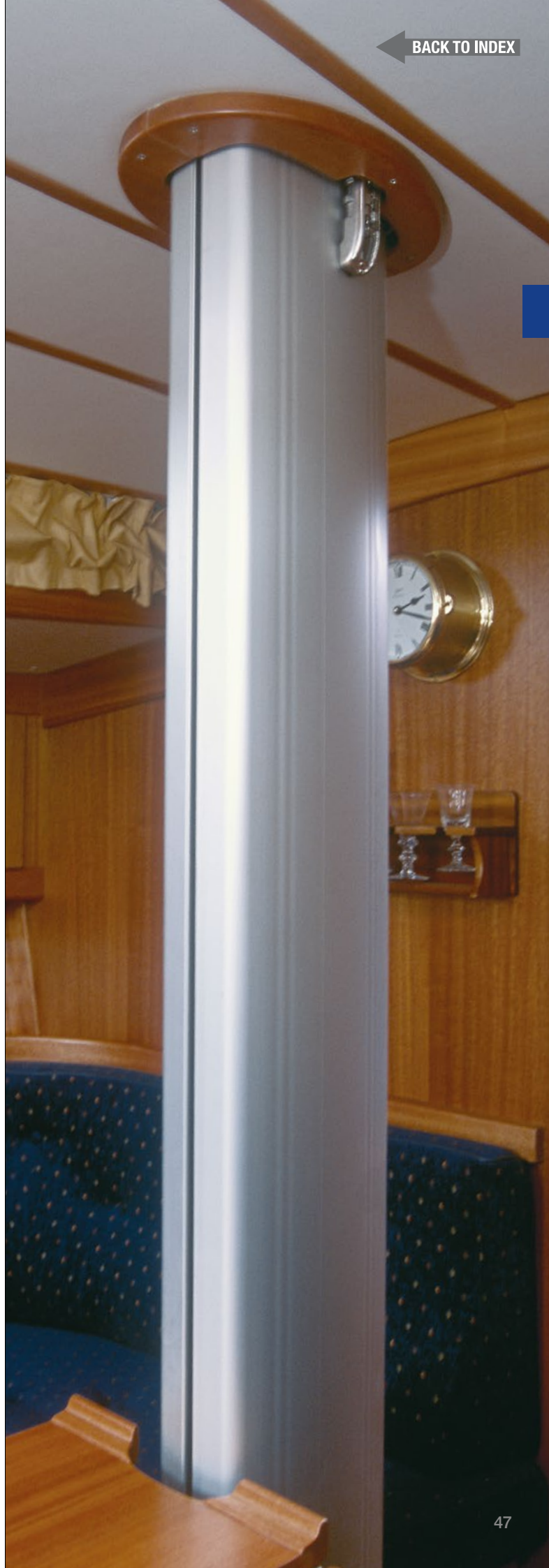
Deck ring with moulded mast coat.
