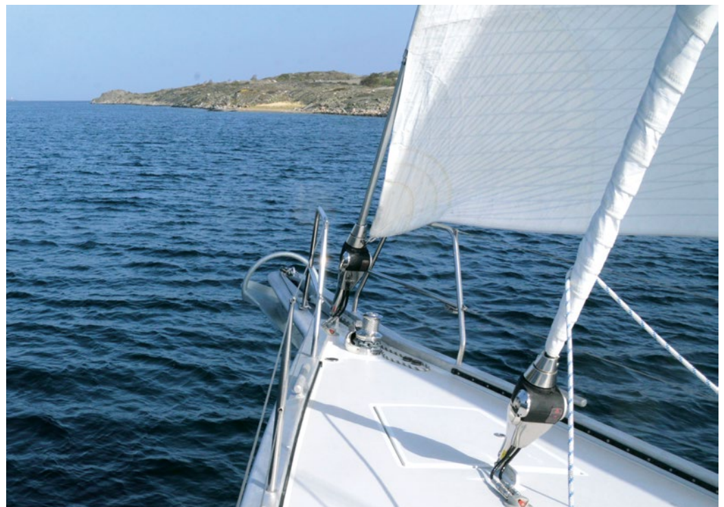
Furlex Hydraulic, deck gland and deck gland protection.
