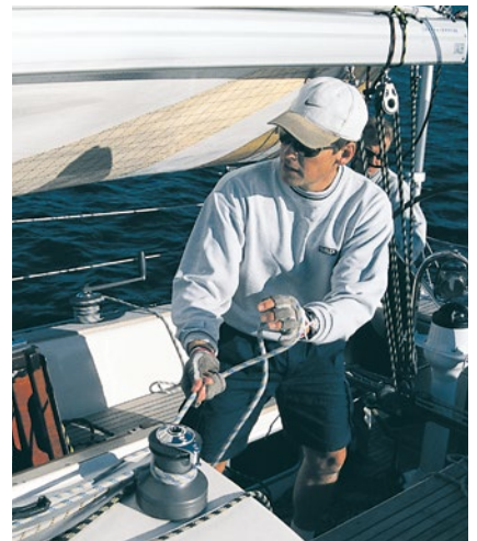
If necessary, apply more main halyard tension.
