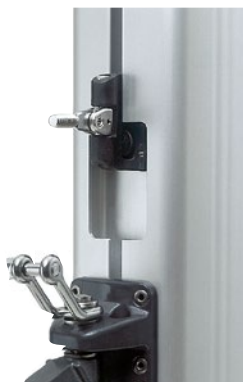
Sail entry gate easily removed to fit or remove Seldén MDS cars.
