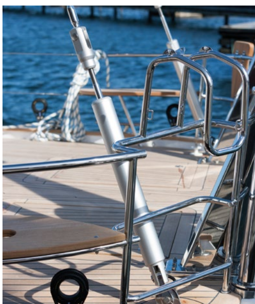
Hydraulic backstay tensioner (HT), operated from a control panel
