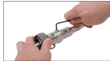
Install the drum/halyard swivel and tighten the locking screw.
