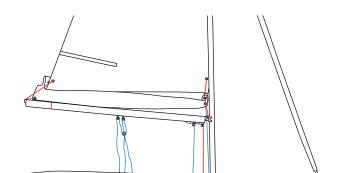
Tension the reef line up to the marked position on the line.
